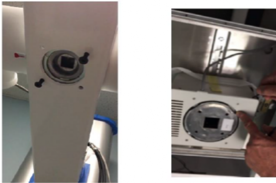
Figure 8: showing the 4 mounting holes at the bottom of the arm to mount the tube and the collimator ring
